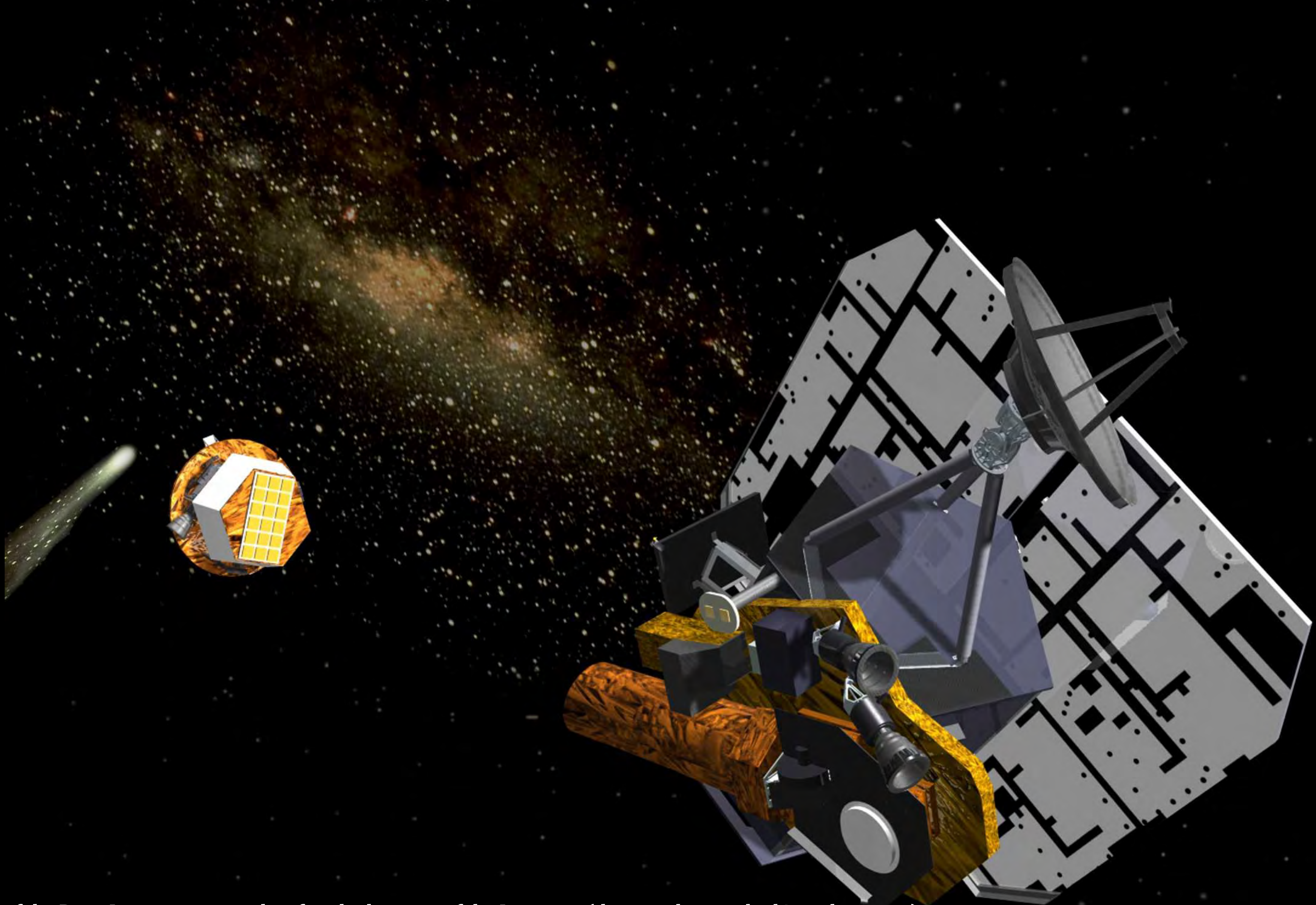
Artist's impression of the Deep Impact space probe after deployment of the Impactor (the part that crashed into the comet)
